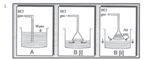
ii. Prevents or minimizes back – suction of water and Provides a large surface area for the absorption of HCl gas
